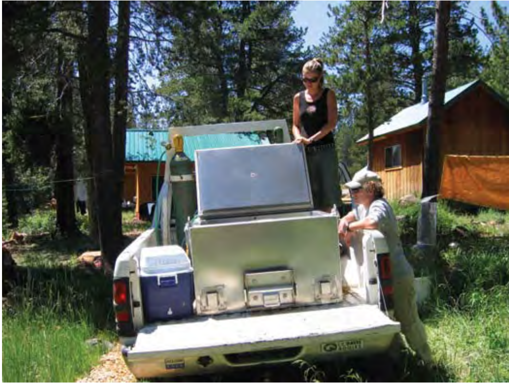
(a) A pickup truck adapted for hauling fish, with an approximately 210-gallon aluminum tank.
